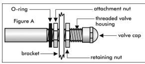
1. Attach one of the valve extenders to the inside wheel valve stem. Be careful not to cross-thread the fittings.
